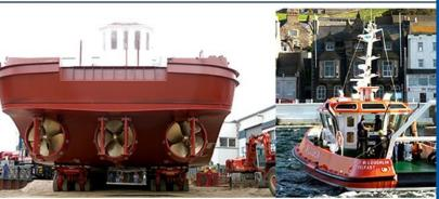
An owner can work his existing fishing gear using less engine power than is needed with an open propeller, resulting in reduced fuel consumption. We have reports from skippers showing 12-20% fuel saving, depending on method of operation and the time spent steaming to and from the grounds.
